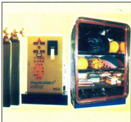
Nitrogen Fumigation Chamber
