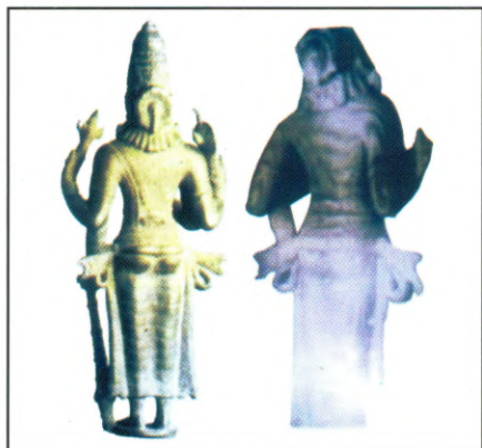
Ordinary Photograph and Fringe Pattern of a Bronze Image
