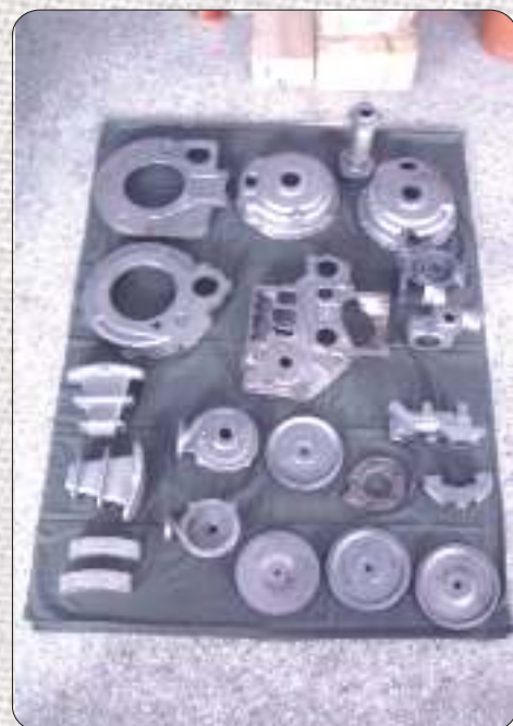
Modern Investment Casting Components based on Lost Wax Technology
